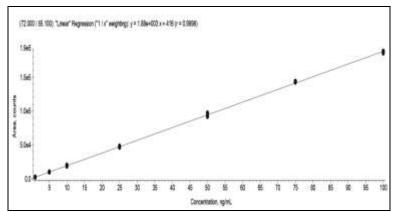
Figure 1. Calibration curve of acrylamide standarts (0.1, 5.0, 10.0, 25.0, 50.0, 75.0 and 100.0 ppb)
